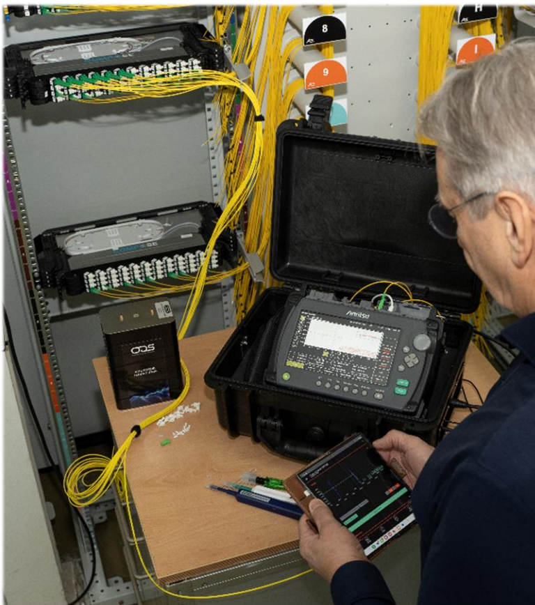
Figure 4: Patching the cloudOTDR plug-in using a launch fiber stack.
